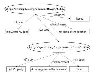
Figure 2. Using an Element
