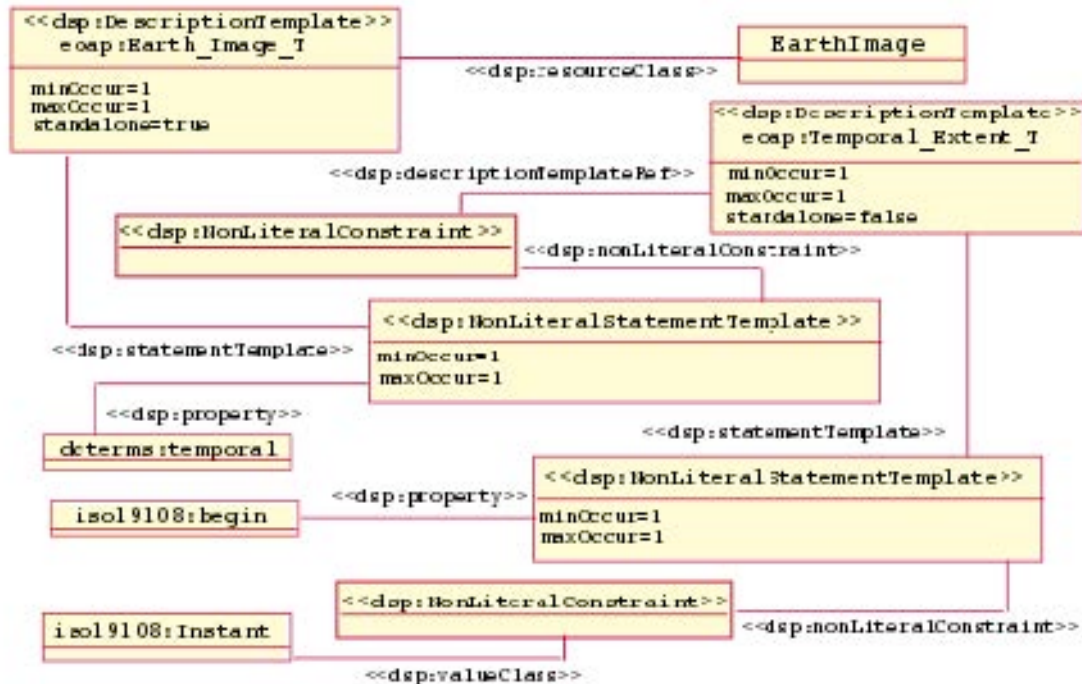
FIG. 3: Short excerpt of the EOAP model as a DSP profile instantiation
